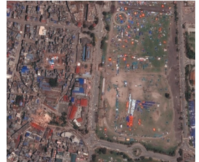
Subscene of Pleiades image of 27 April 2015 over Kathmandu (48 hours after the earthquake) showing the collapsed Dharahara Tower (bottom left) and emergency tents in the park.
