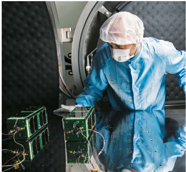
The Ecole Polytechnique's XCubesat and the Ecole des Mines' Spacecube in the thermal vacuum chamber at the integration and test platform at the University of Versailles Saint-Quentin-en-Yvelines (UVSQ).
